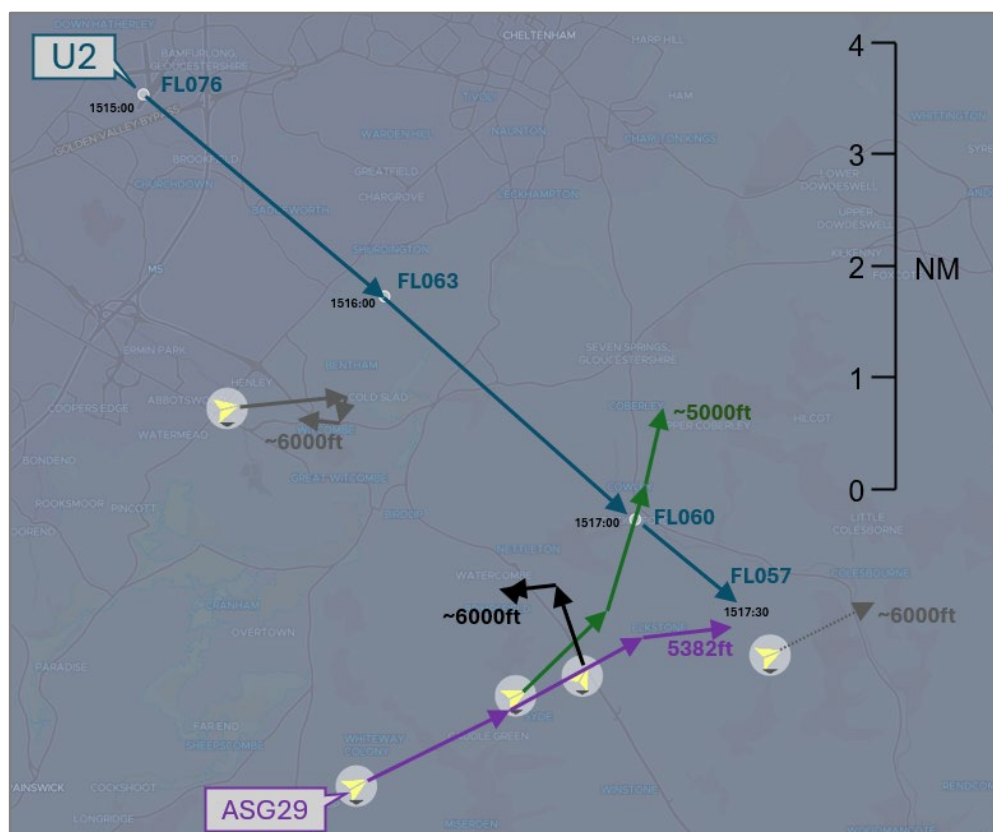
Figure 3 – The traffic situation at 1515 (radar and FLARM data). The arrowheads indicate respective positions at 1516, 1517 and 1517:30
