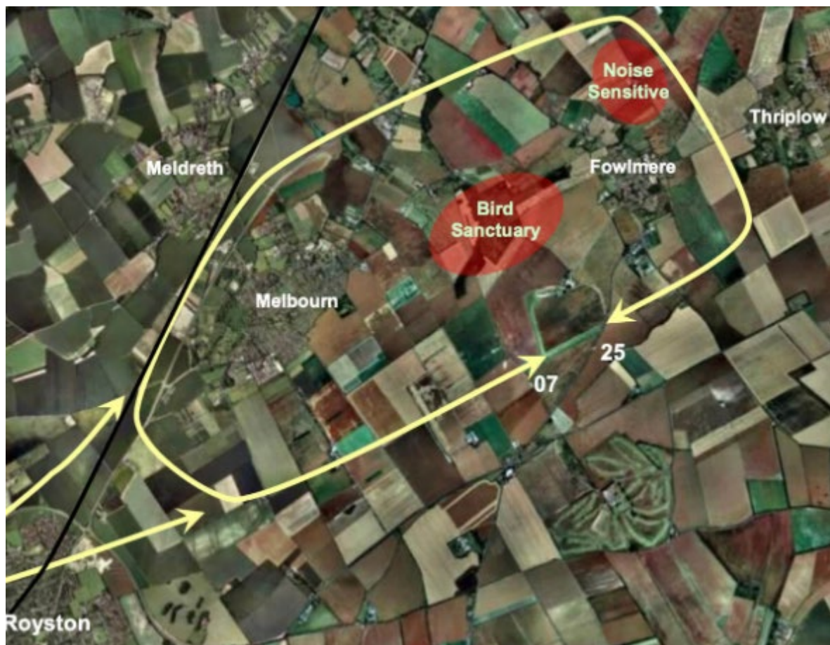
Figure 1 – Fowlmere Visual Circuit diagram.
