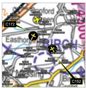
Figure 2: From the CAA's Airspace analyser Tool at 1207:00. The C172 is shown to be at 1388ft/029°/90kt/0fpm and the C152 (the last time the C152 data refreshed had been at 1206:20) at 1625ft/328°/101kt/-700fpm. The orange dot shows the CPA.
