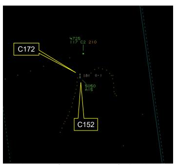
Figure 1: At CPA 1206:59 ~110ft V/0.1NM H
