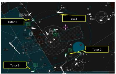
Figure 1 (1332:02). Traffic Information provided to the pilot of Tutor 3. (Separation: Tutor 1 to BE33 2.9NM)
