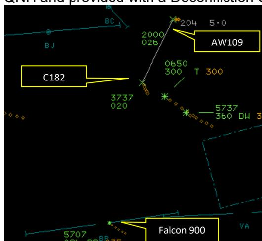
Figure 2 (1233:38). Separation between the C182 and AW109 fell below 5NM laterally.
