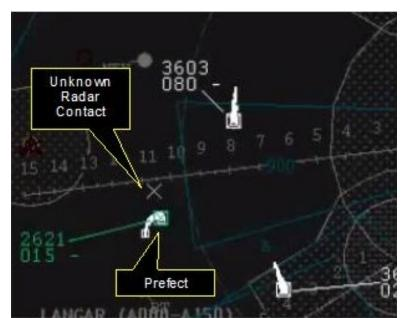
Figure 2 (1237:59). Unknown radar contact displayed. Separation estimated as 1.0NM
