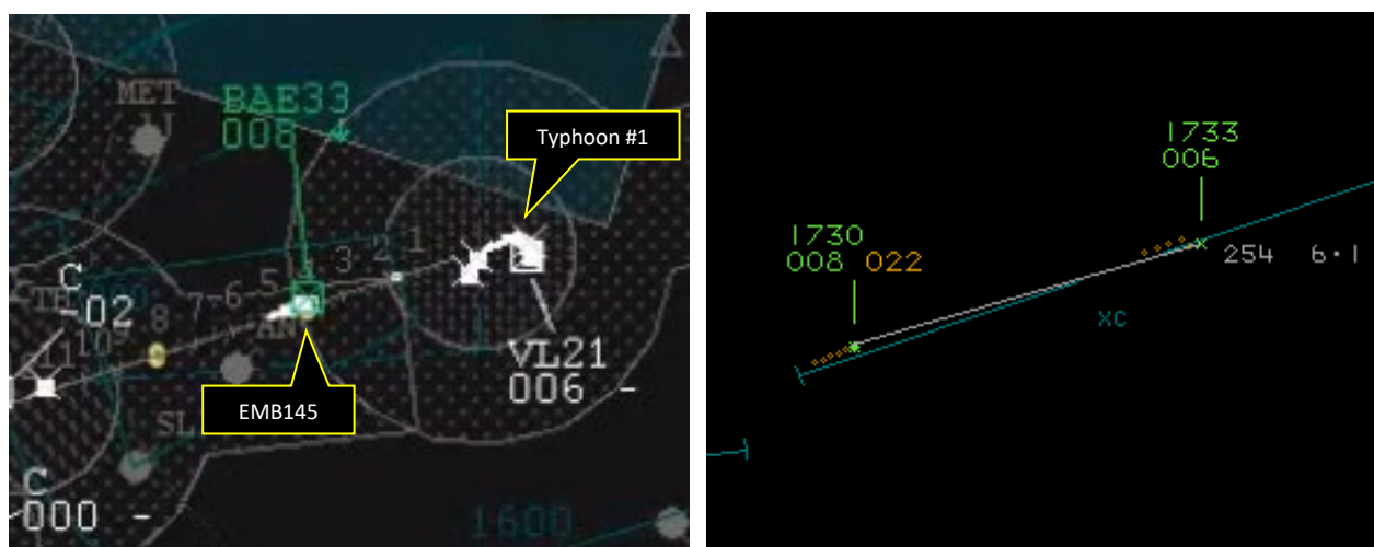
Figure 2 (1425:12). The Coningsby Surveillance Radar Approach controller broke off the EMB145 in accordance with the Coningsby Tower controller instruction. (Separation 6.1NM)
