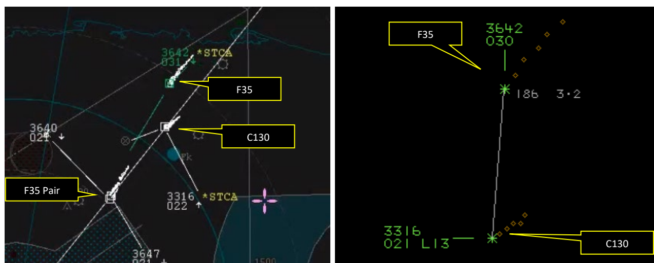
Figure 3 (0900:22): Short-Term Conflict Alert (STCA) received by both the Marham Approach controller and Marham Zone controller. (Separation 3.2NM) (unit radar left, NATS radar right)
