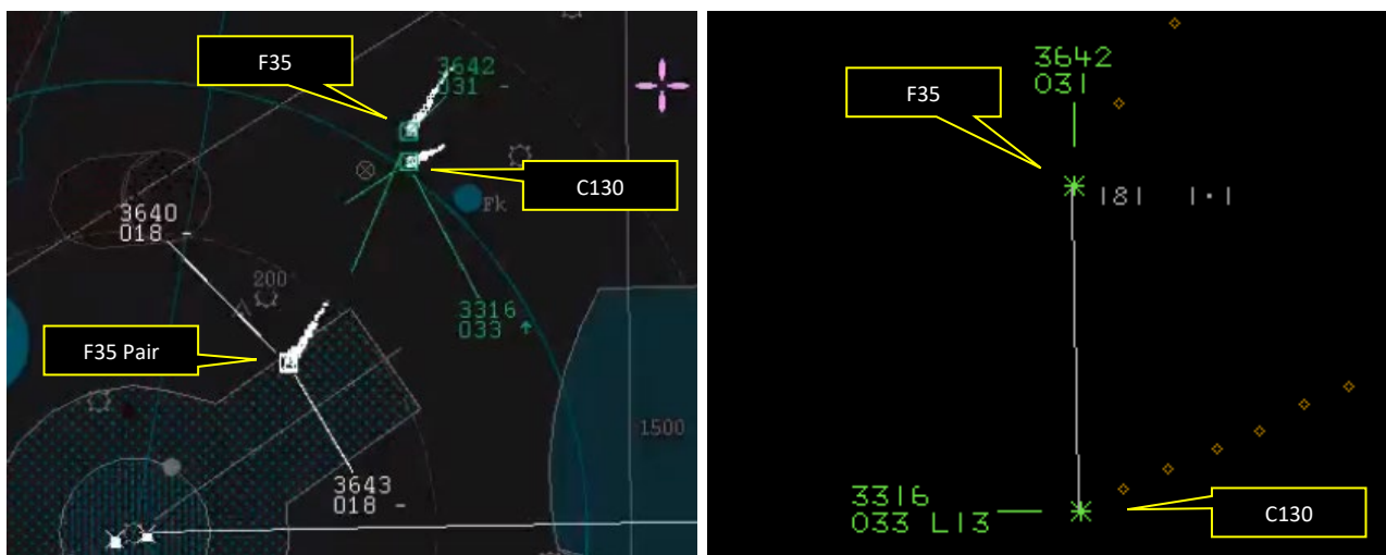
Figure 4 (0900:58): Updated Traffic information provided by the Marham Approach controller. (Separation 1.1NM) (unit radar left, NATS radar right)
