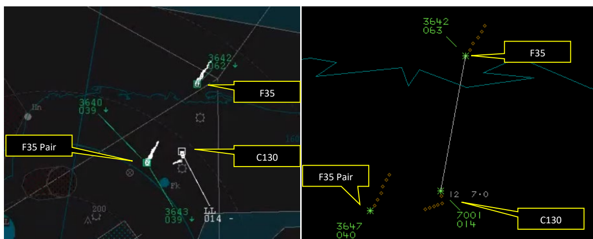
Figure 2 (0859:18): Updated Traffic information provided by the Marham Approach controller. (Separation 7.0NM) (unit radar left, NATS radar right)
