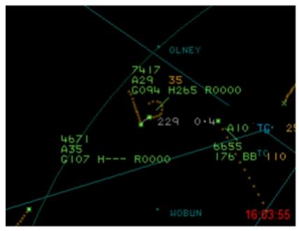
Figure 1 - CPA measured on the Multi-Track Radar as 0.4NM and 600ft.
