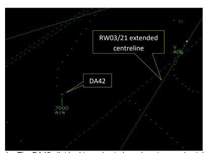
Figure 1 – The DA42 pilot had turned onto base-leg at approximately 1417
