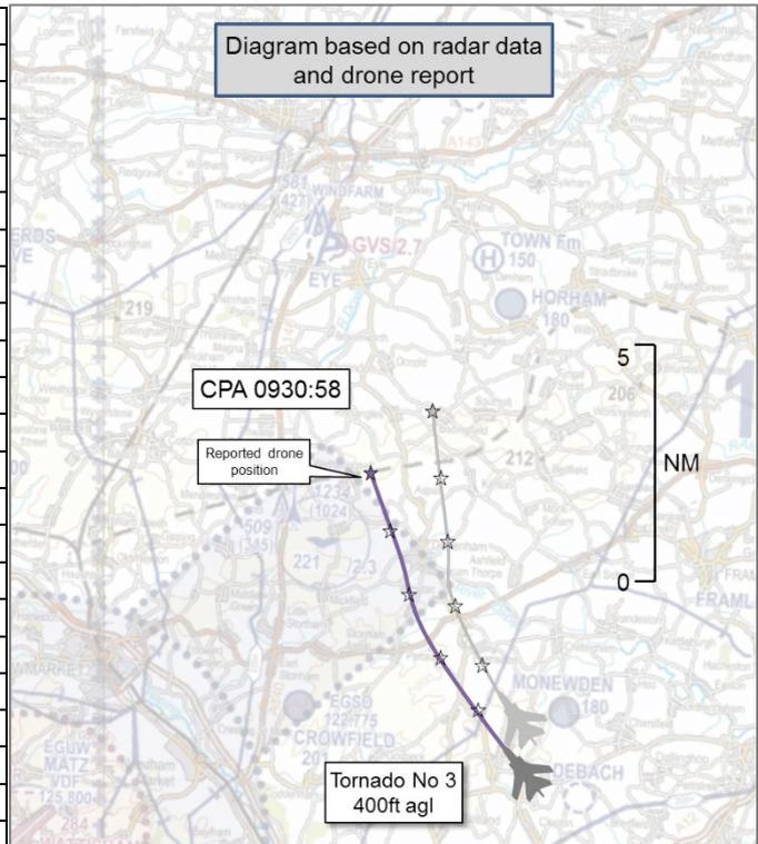
**THE DRONE OPERATOR** reports carrying out an agricultural survey. Whilst the drone was heading south on a return leg, a Tornado passed from behind at high speed over the same field, heading north. The drone was put into a rapid descent, by which time the Tornado had passed the field.
