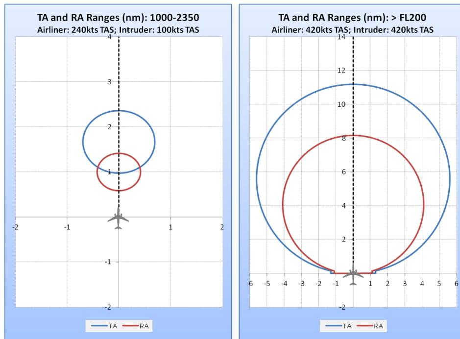
**Figure 21. Representative TCAS TA/RA envelopes (note the different scales for each diagram)**
