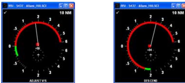
The simulated IVSI above shows that, at the time of the initial “Adjust Vertical Speed” RA, the BE200 was climbing at approximately 1600ft/min and that the RA required a negative vertical rate. By the time of the subsequent “DESCEND” RA the aircraft’s RoC had increased to 2500ft/min, while the RA now required a rate of descent of not less than 1500 ft/min.
