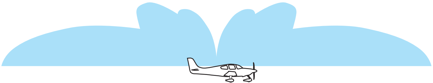
The theoretical coverage provided a top fuselage-mounted monopole antenna.
