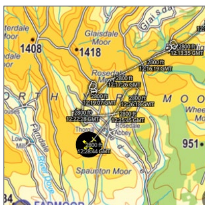
Figure 3: from the CAA's Airspace Analyser Tool - G109 showed for the last time ~0.5NM short of CPA at 1229:00 at 2800ft (SPS).
