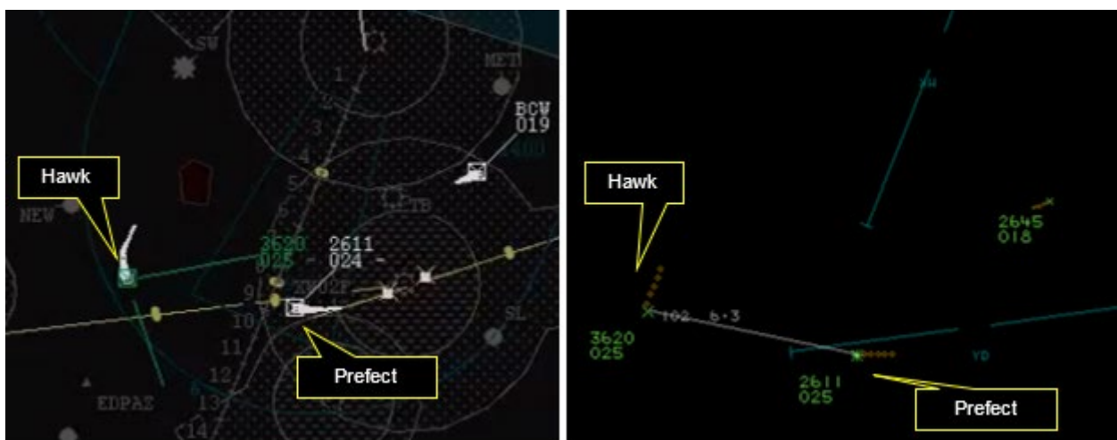
Figure 4 (1336:57) - Traffic information provided to the Hawk [pilot] on the Prefect. Separation: 6.3NM
