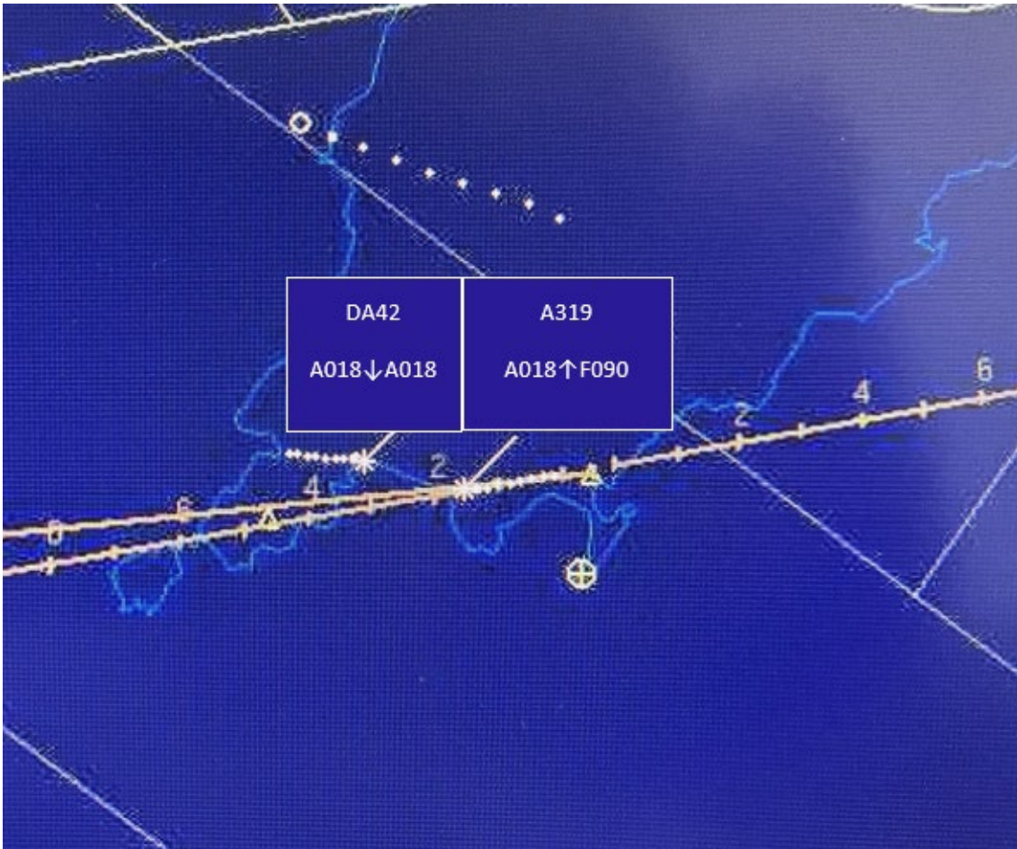
Figure 1 - 1022:00. The A319 appeared on the radar screen co-alt with the DA42.
