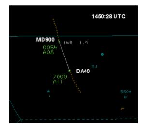
At 1450:56 the position indication symbols of the ac merged on the radar replay with the MD900 at altitude 900ft and the DA40 at altitude 1200ft (as shown below).
