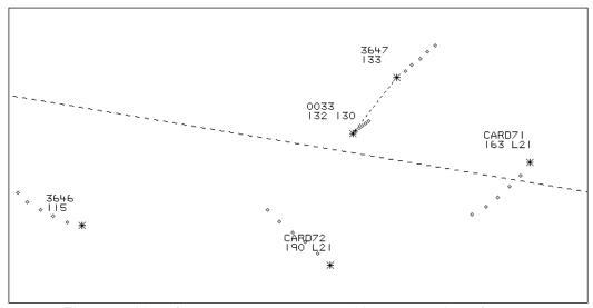
Figure 4: Aircraft geometry at 1224:42 with a separation of 1.7nm
