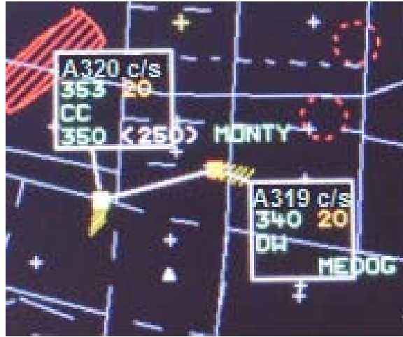
(Figure 7 – STCA alert after the T controller moved the A320 label - 1732:23)
