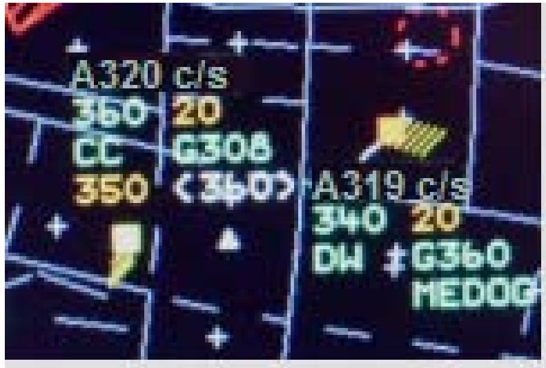
(Figure 4 – iFACTS alert showing A320 CFL as 350 and SFL as 360 – 1731:03)
