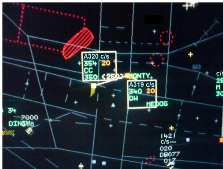
(Figure 6 –STCA activates at 1732:15 – vertical separation is 1400ft)
