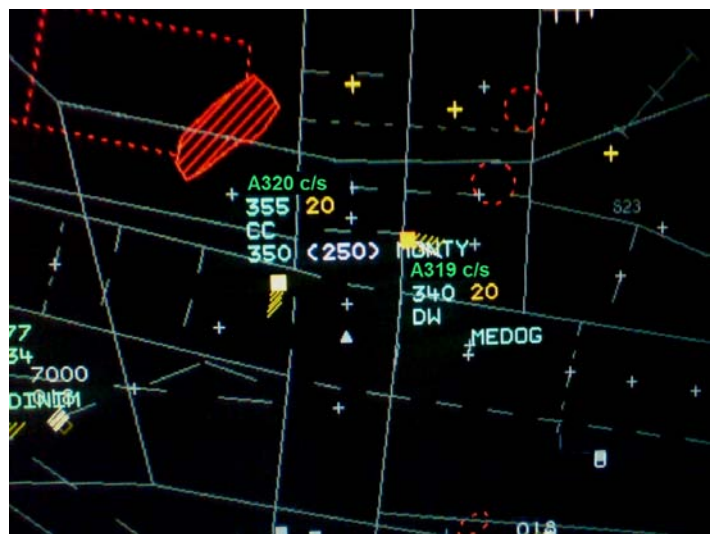
(Figure 5 – iFACTS alert showing A320 CFL as 350 and SFL as 250 - 1731:55)
