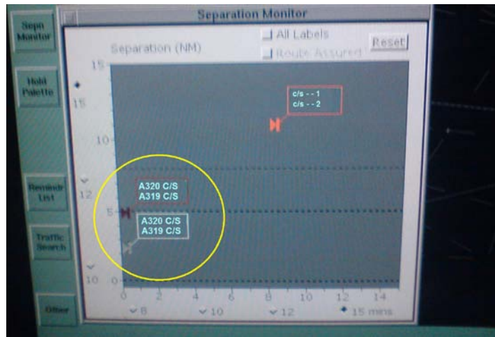
(Figure 9 – iFACTS separation monitor interactions - 1732:52)
