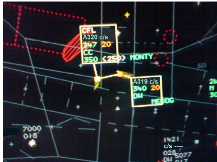
(Figure 8 - STCA, the CFL deviation alert and incorrect SFL alert - 1732:52)
