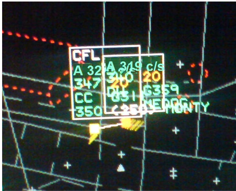
(Figure 10 – Overlapping labels on the P controller's situation display - 1732:52)
