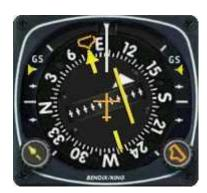
Figure 1. Example Heading Indicator
