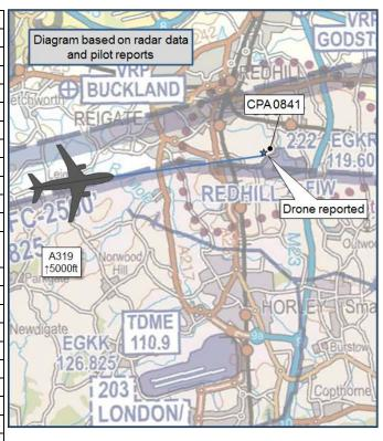
**THE A319 PILOT** reports that the aircraft was on a easterly heading on the ADMAG1X departure from Gatwick. On passing about 5000ft, the second officer noticed a small, blue object (which looked like a drone), fly very close to the aircraft. It flew less than 100ft under the wing of the aircraft, its track taking it between the fuselage and the number 2 engine. No avoiding action was taken because the object was not seen until very late. It was reported to ATC immediately.
