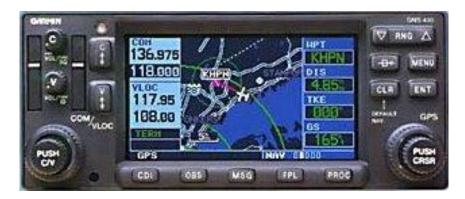
Figure 1 – Example Garmin 430 Navigational Display.<sup>1</sup>
