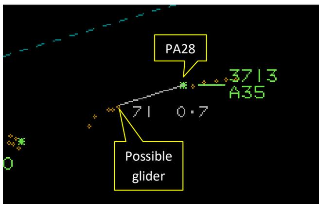
Figure 2 – Primary contact fades from radar
