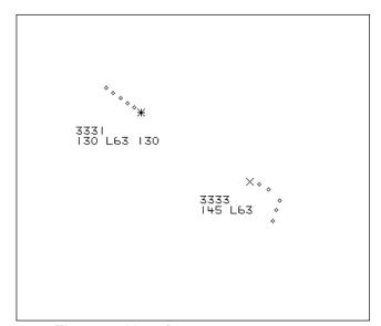
Figure 2: Aircraft geometry at 1205:04.
