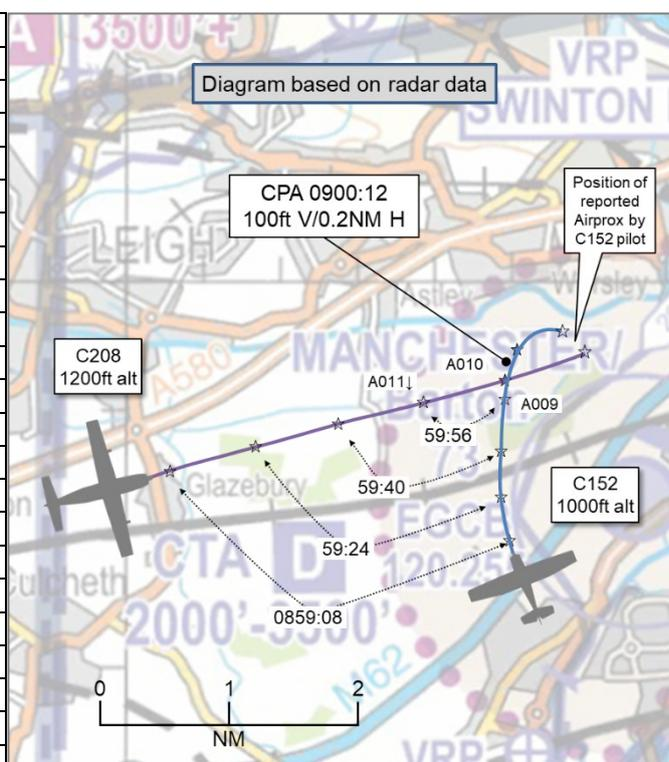
**THE C152 PILOT** reports that they were flying downwind on a circuit detail at Barton. The C208 [pilot] joined behind them, having made a late radio call. The C208 pilot proceeded to undercut them at a much greater speed, with very limited separation.
